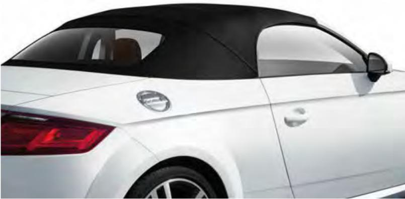
Quality enhanced, exterior noises reduced: the fully automatic acoustic hood made from insulated 3-layer fabric captivates with its high-quality covers in three different colours. It can be opened and closed at speeds of up to 50 km/h in 10 seconds and ensures a pleasantly quiet ride as well as excellent heat insulation.
